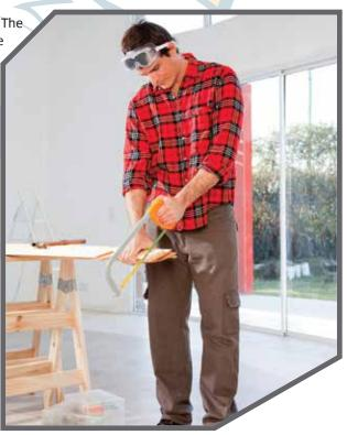
You cut with the hacksaw using long strokes that utilize the entire blade length, releasing pressure on the blade on the backward stroke. There is no cutting that takes place on the back stroke, so maintaining pressure only tires you out and shortens the blade life.
